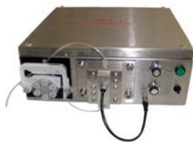
Installation of a dynamic image analysis with software for particle size and shape analysis
